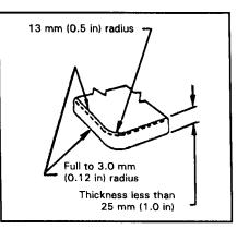
b. Exposed corners 25 mm (1.0 in) thick or greater shall be rounded to 13 mm (0.5 in) spherical radius, as shown in Exhibit 12.5.1.5 (b). [Source: NASA-STD-3000A, 1989]
