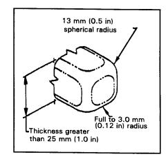
12.5.1.6 Projecting components. In areas where maintainers must make rapid movements, small projecting components should be avoided or covered. [Source: MIL-HDBK-759B, 1992]
