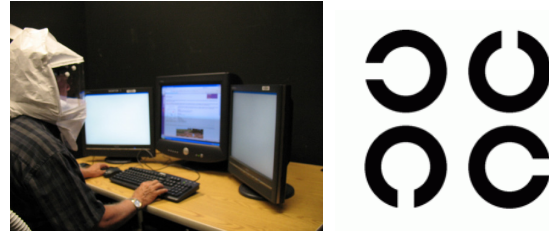
Figure 4. Visual performance task set up (left) and the Landolt C in four orientations of the opening (right).
