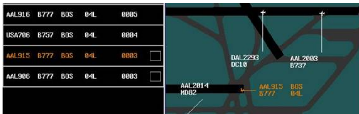
Figure 23. An aircraft that has taxied into position and is holding on the runway causing highlighting of the aircraft's FDE and data block.
