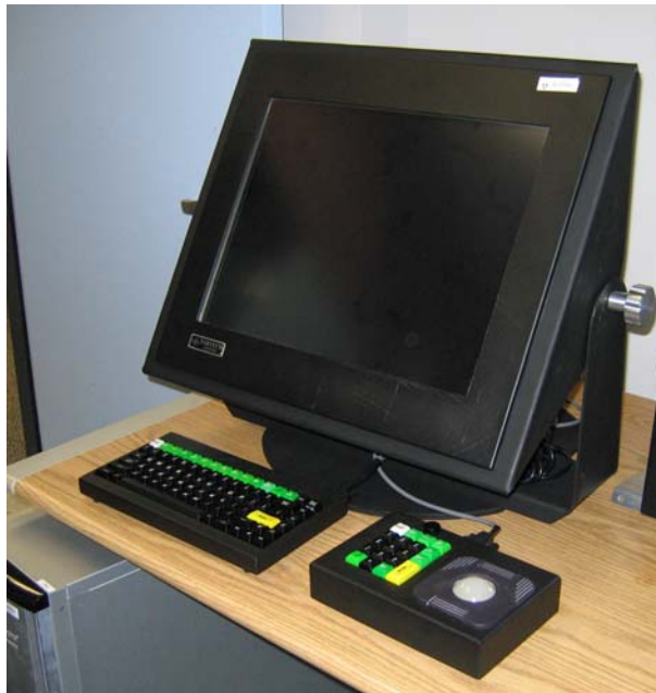
Figure 1. Hardware used to implement the prototype Integrated EFDI including resistive touch display, display mount, ASDE-X keyboard, and trackball/keypad.
