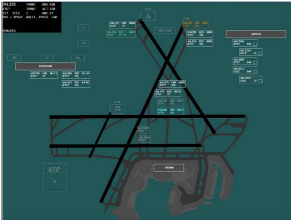
Figure 25. The primary elements of the P-S EFDI including FDEs, the readout area, buttons, and system information window.
