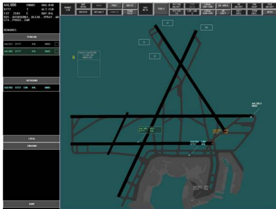
Figure 2. The primary elements of the ground controller's Integrated EFDI including the surface situation display, EFD lists, and readout area.
