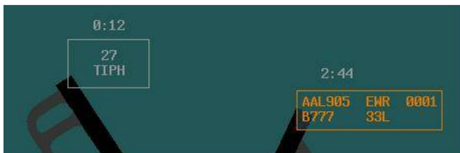
Figure 29. Unoccupied and occupied TIPH buttons for two intersecting runways.
