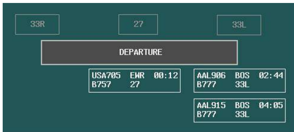
Figure 31. FDEs for aircraft that the local controller has cleared for departure appearing in the departure list on the local control P-S EFDI.
