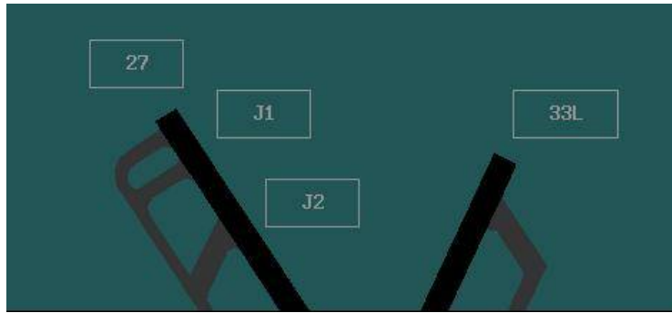
Figure 16. Buttons on the Integrated EFDI situation display for runway and intersection departure assignments.
