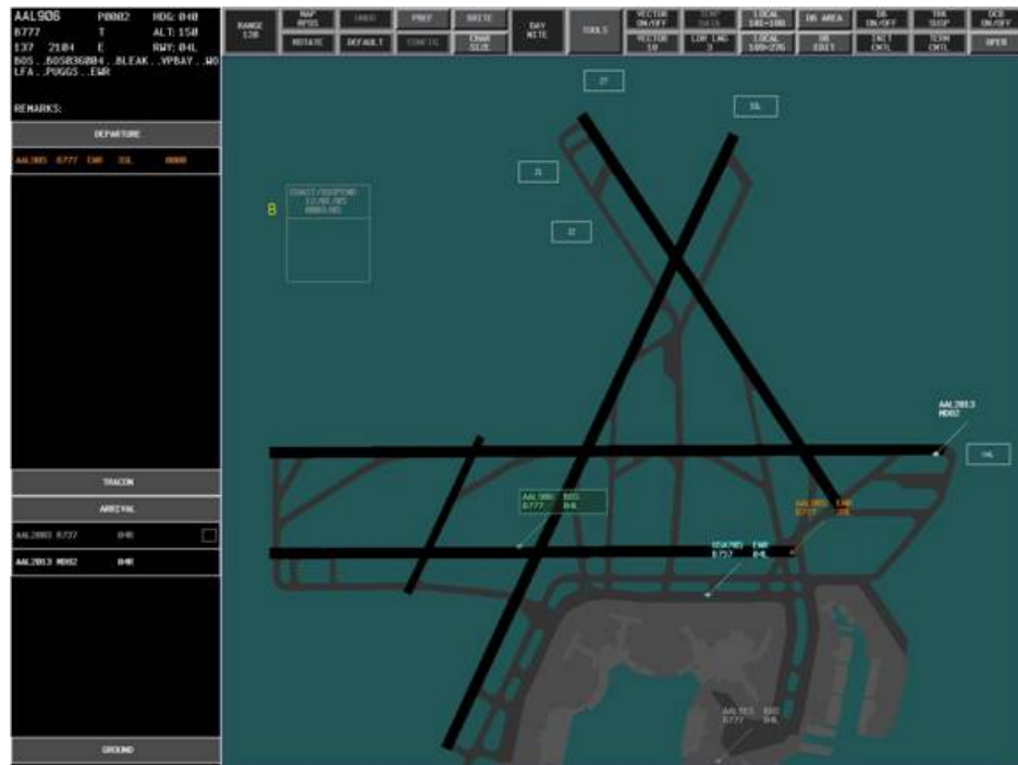
Figure 3. The primary elements of the local controller's Integrated EFDI including the surface situation display, EFD lists, and readout area.
