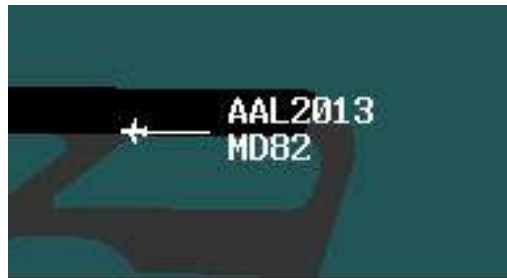
Figure 11. Arrival aircraft position symbol, leader line, and data block on the local control Integrated EFDI.
