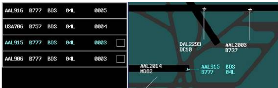
Figure 22. A highlighted FDE and the associated data block.
