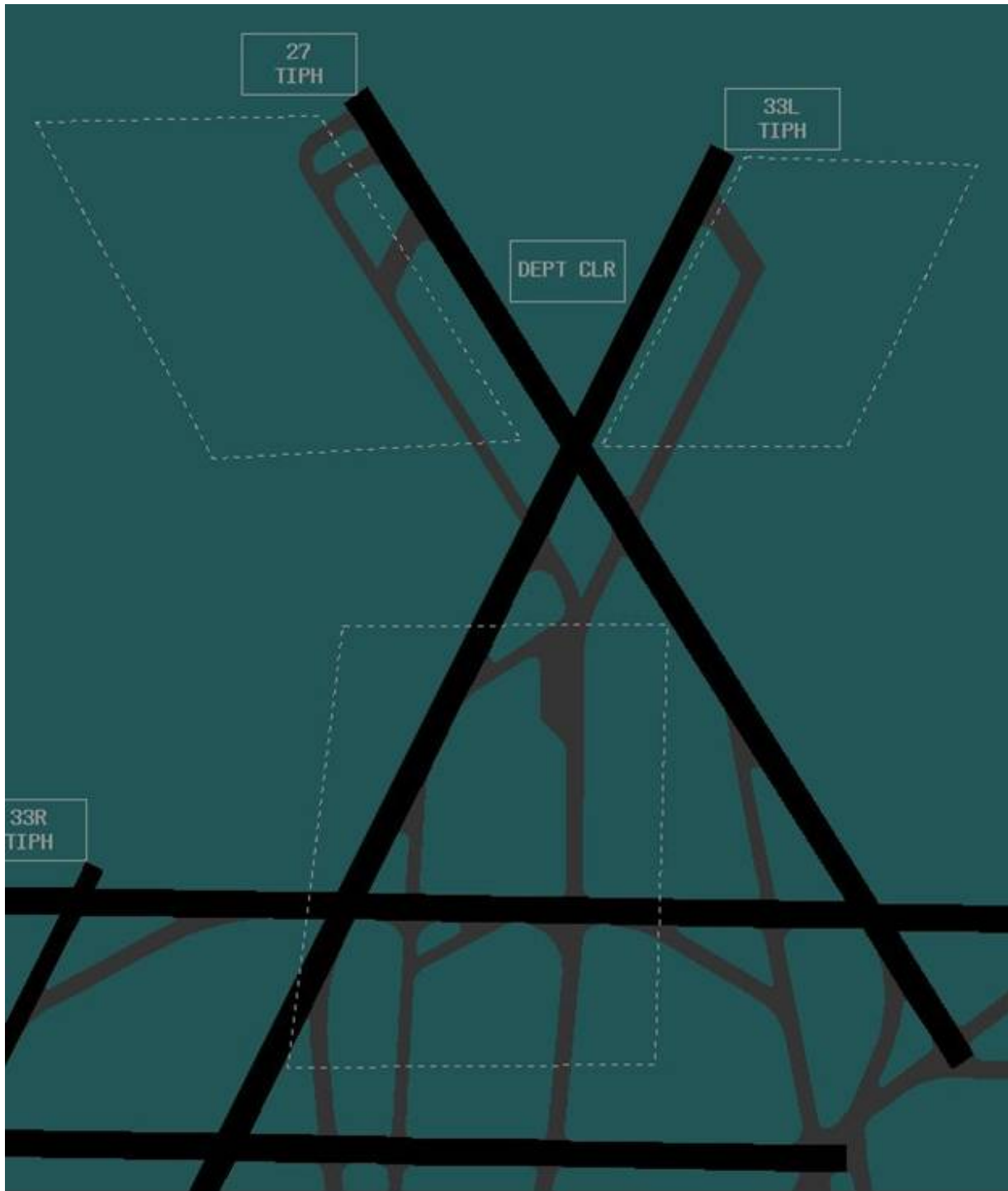
Figure 34. FDE zones on the local control P-S EFDI.
