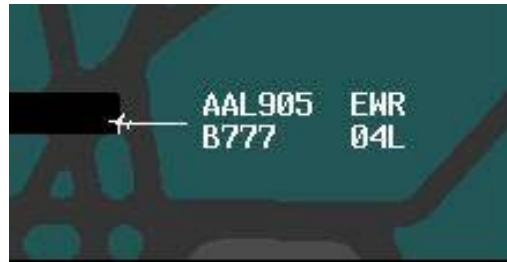
Figure 10. Departure aircraft position symbol, leader line, and data block on the local control Integrated EFDI.
