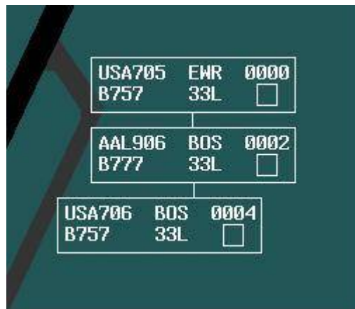
Figure 28. Departure FDEs on the local control P-S EFDI showing the flight data attributes.
