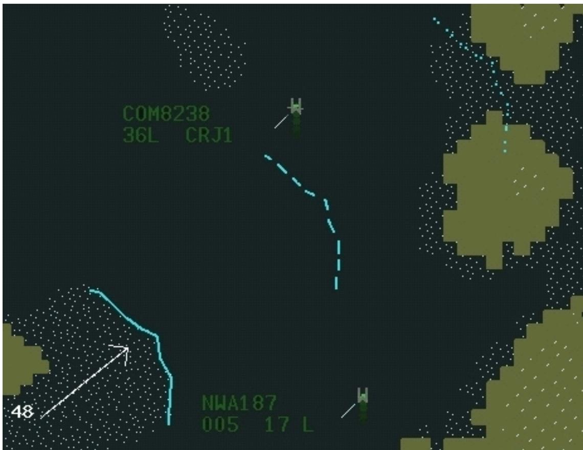
Figure 2. Illustration of the static Storm Motion tool. The vector (arrow) indicates the direction of cell motion, and the numerals indicate the cell speed in knots. The solid blue line depicts the storm cell leading edge, the broken blue line depicts the 10 minute extrapolated position, and the dotted blue line depicts the 20 minute extrapolated position.
