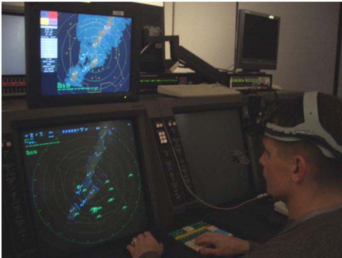
Figure 1. Simulation setup with the STARS controller workstation (bottom) and the WIDS display (top). The researcher in the figure is wearing the Applied Sciences Laboratory Series 6000 Model 501 eye and head tracking system used during the simulation.
