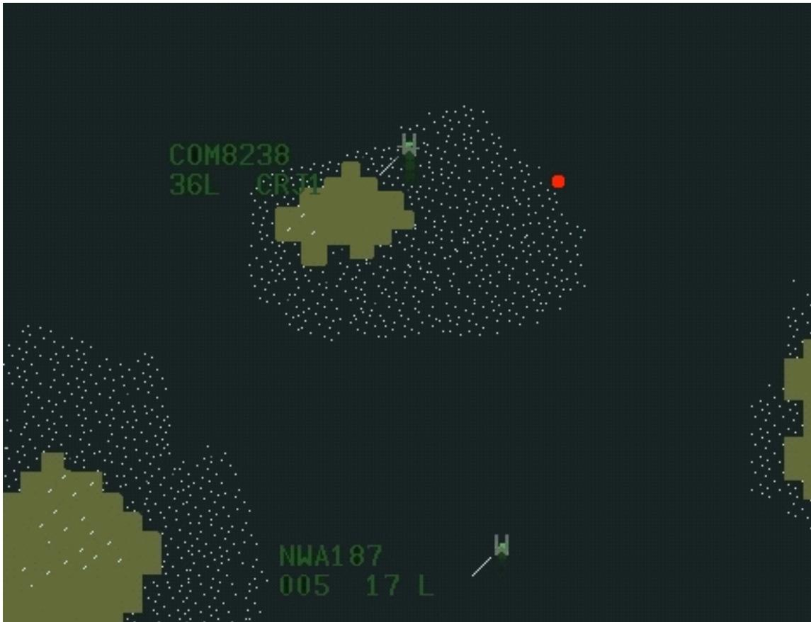
Figure 4. An illustration of the Dynamic Storm Motion tool after activation. The leading edge of the storm cell (red dot) together with all selected precipitation areas (solid and dotted areas) are extrapolated to a position 15 minutes into the future.
