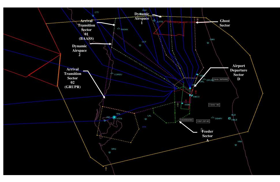
Figure 3. A chart of the airspace for the Big Airspace conditions.
