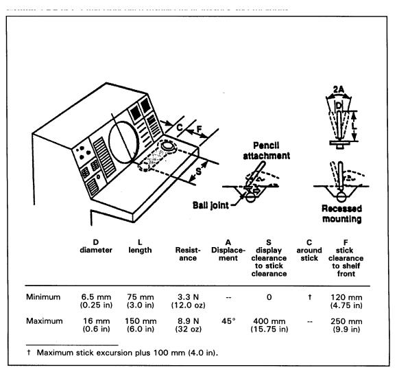
Exhibit 9.3.3.3.1 Finger-operated displacement joystick specifications
