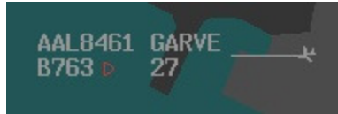
Figure 15. Data link indicator showing a failed data link transmission.
