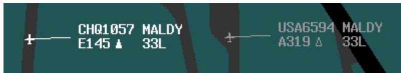
Figure 4. Data link capability indicators for owned (left) and unowned (right) aircraft.
