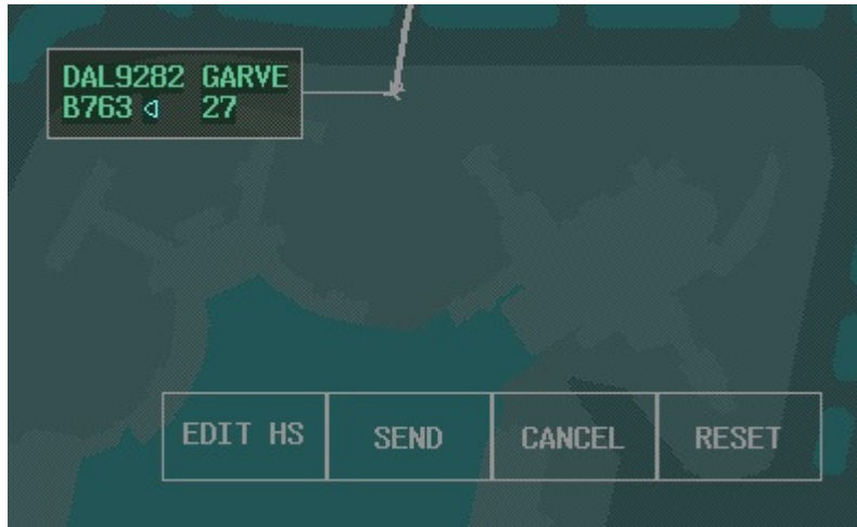
Figure 10. Selected data block and D-Taxi construction mode buttons.
