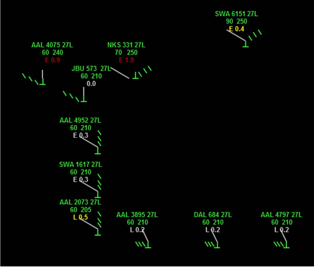
Figure 6. Close-up view of prototype P-GUI display with E/L indicators, fractions of minutes, and color coding.
