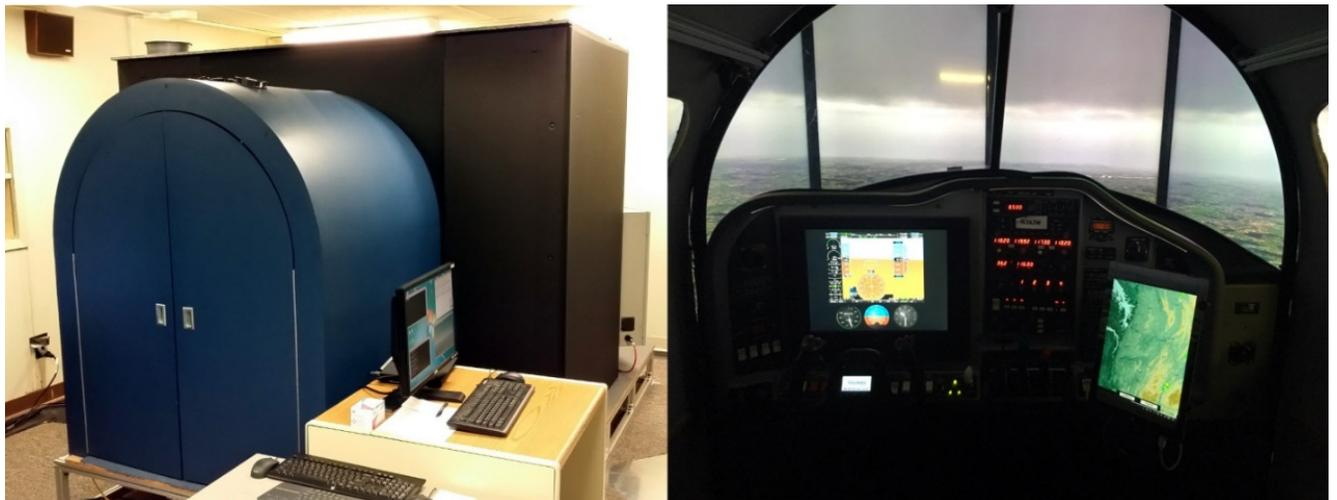
*Figure 1.* Left: an exterior view of the MicroJet fuselage. Right: the cockpit out-window view, the G1000 type GA glass cockpit control display, the instrument (radio) stack, and the stand-alone weather display running on a Windows Surface Pro 3.
