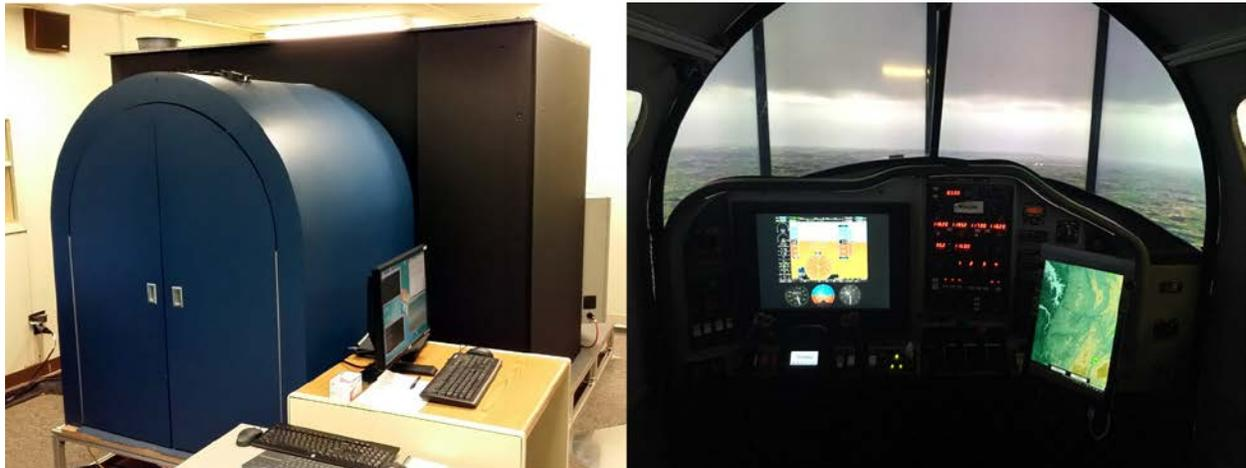
Figure 2. Left: an exterior view of the generic GA aircraft fuselage. Right: the cockpit out-the-window view, the G1000 type GA glass cockpit control display, the instrument (radio) stack, and the stand-alone weather display running on a Windows Surface Pro 3.
