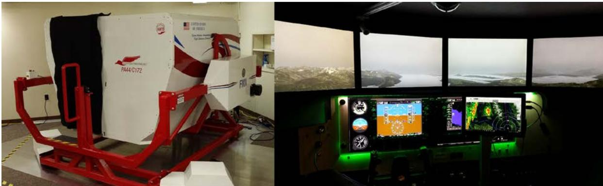
Figure 27. Left: an exterior view of the Redbird C172 fuselage. Right: the cockpit out-window view, the G1000-type GA glass cockpit control display, the instruments, and the stand-alone weather display running on a Windows Surface Pro 3.
