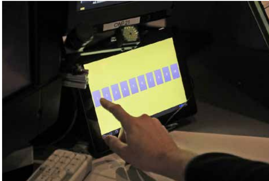
Figure 6. Workload Assessment Keypad (WAK)
