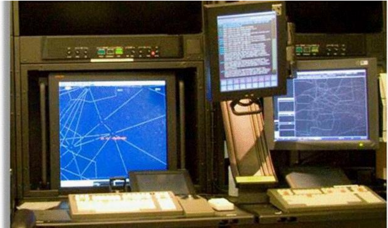
Figure 9. ERIDS console mounted on a moveable arm between the radar and radar associate position.
